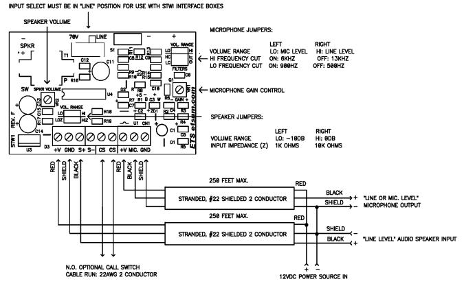
LINE/MIC. MICROPHONE OUTPUT AND LINE LEVEL SPEAKER INPUT
