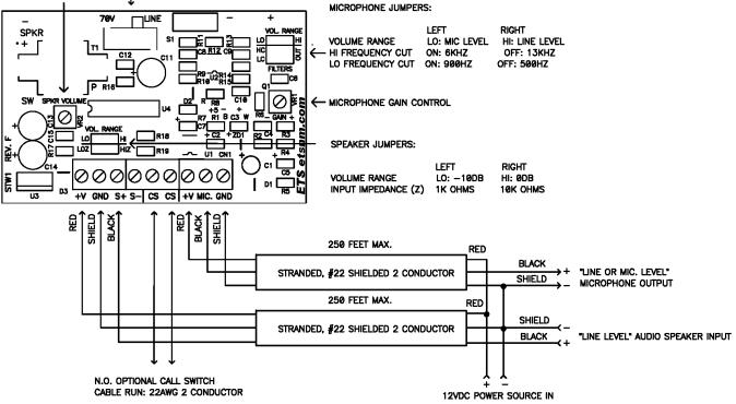
INPUT SELECT MUST BE IN "LINE" POSITION FOR USE WITH STWI INTERFACE BOXES
